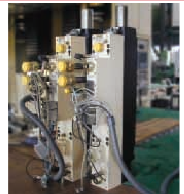
Two out of 16 hydraulic cushion cylinders with directly flanged control block: Pressure, tank and control lines are mounted directly.
