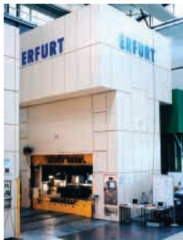
Try-out presses appear to be “top heavy” since a major part of the hydraulic control units are installed in the upper part of the press and hence close to the consumers.
